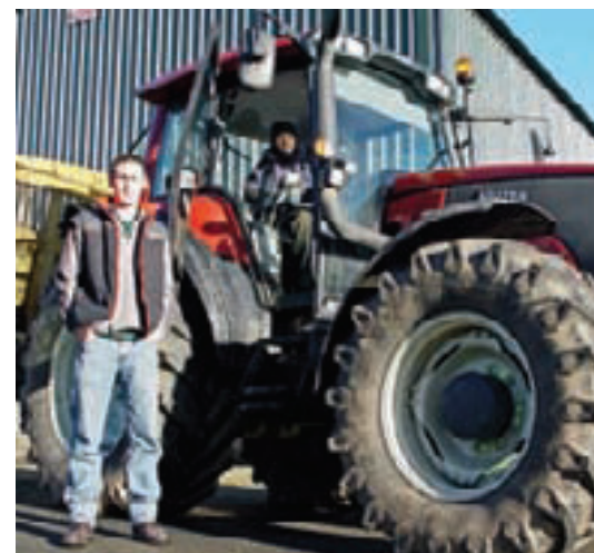
Richard Piggott discusses the day's work with a driver; All TES tractors operate with O licences, have front suspension and air brakes to the trailer or spreader.
